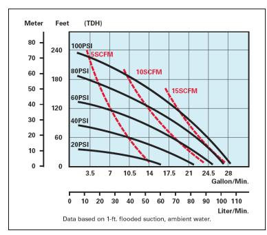
The performance curves shown and other published literature reflect an average performance for all materials and all elastomers, including Teflon<sup>®</sup>. Derating of the performance is not necessary for Teflon<sup>®</sup> fitted pumps.
