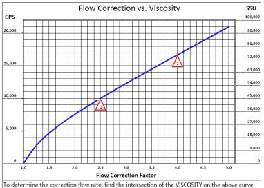
and use this new flow rate to select a pump from the performance curves.
